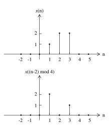
Figure 1: Right Circular Shift on x[n] = [0, 1, 2, 2] by 2 points
