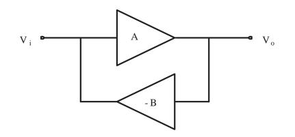
Figure 1: Typical negative feedback
