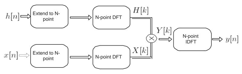
Figure 2: Flow Diagram
