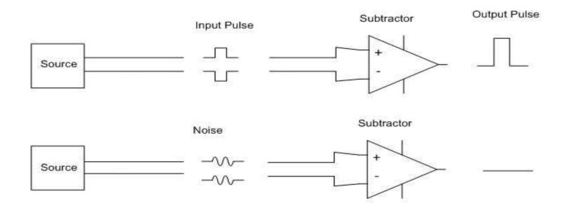
Figure 3: A differential receiver setup
